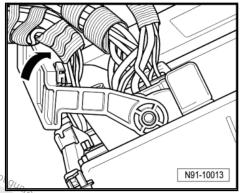
Release connectors -arrows of aerial connections and disconnect connectors.
