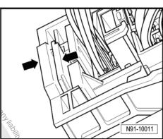
Sen suit Then swing locking bar up in direction of -arrow- and disconnect connector.
