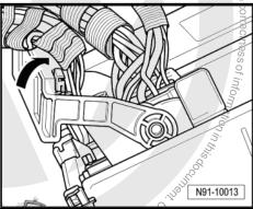
Release connectors -arrows- of aerial connections and dis-Protectedbyo connect connectors.
