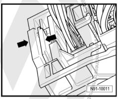
Then swing locking bar up in direction of -arrow- and disconnect connector.
