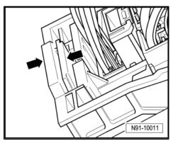
Then swing locking bar up in direction of -arrow- and disconnect connector.
