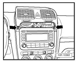
Carefully lever out cover of centre console using removal wedge -3409- -arrows- and take it off.
